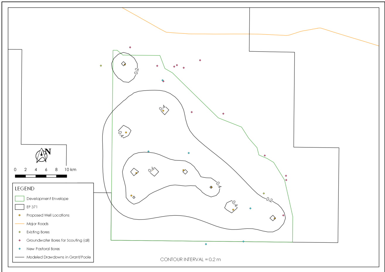
Figure: Mod 2 model results presented as drawdown contours after six months of pumping with contour interval = 0.2 m (Intera model)
