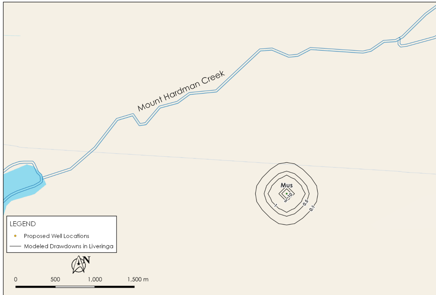
Figure 17-3. Modelled Liveringa Aquifer drawdowns at the proposed Muspelheim abstraction bore as presented in the original model report. Modelled drawdowns are in meters.
