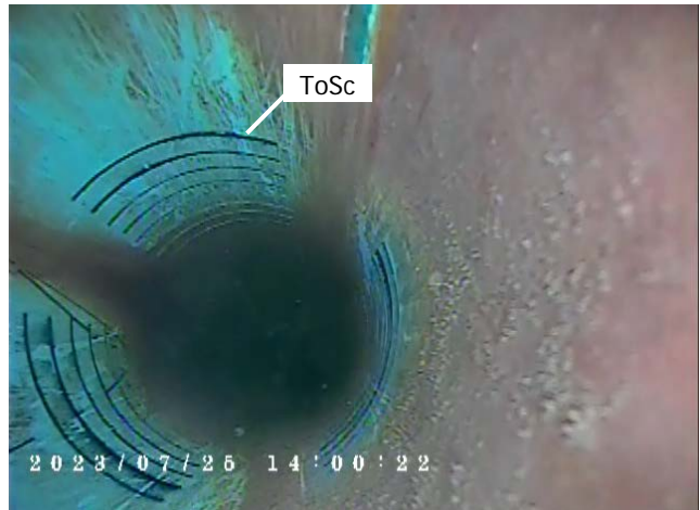
AB1S top of screened interval (ToSc) 30.8 m btoc.
