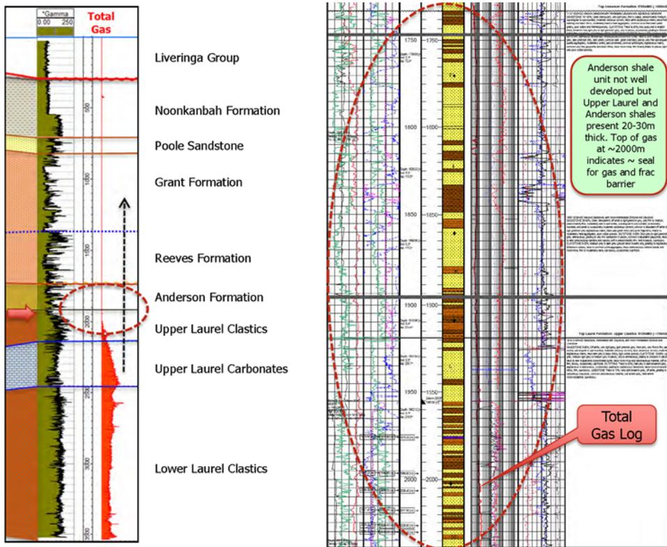
Figure 3-6: Asgard 1 composite well log showing the top of gas in relationship to the upper Anderson and Reeves Formations
