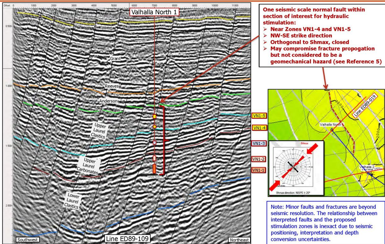
**Figure 3-2: Valhalla North1 – 2D Seismic section showing the detail of the Upper Laurel Formation and faults as well as the relationship to the overlying Anderson, Reeves and Grant Group formations. The base of the Reeves Formation is noted as not a consistent reflector**
