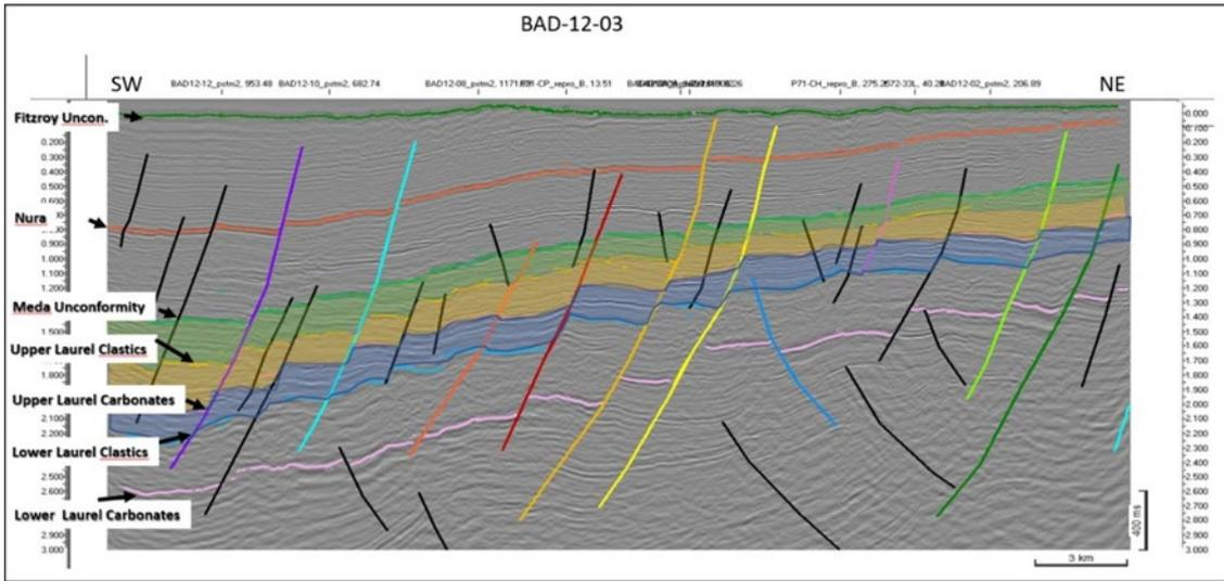
**Figure 2-2: A 2D seismic line in two-way time along the northern edge of the Fitzroy Trough showing the Anderson (Green) and Upper Laurel Formation (Yellow and Blue) benches down stepping into the basin. Some expansion of the Laurel and Anderson Formation sequence is shown. An extensive database of 2D seismic was used to map in three dimensions the structural style of the basin margin. Location of this 33 km long line is shown in Figure 23.**
