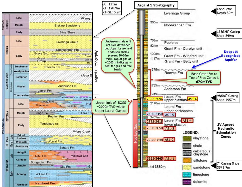
Figure 3-5: Asgard 1 stratigraphic section noting the deepest aquifer and the underlying siltstones of the Reeves and Anderson Formation shales and hydrocarbon zones within the Laurel Formation
