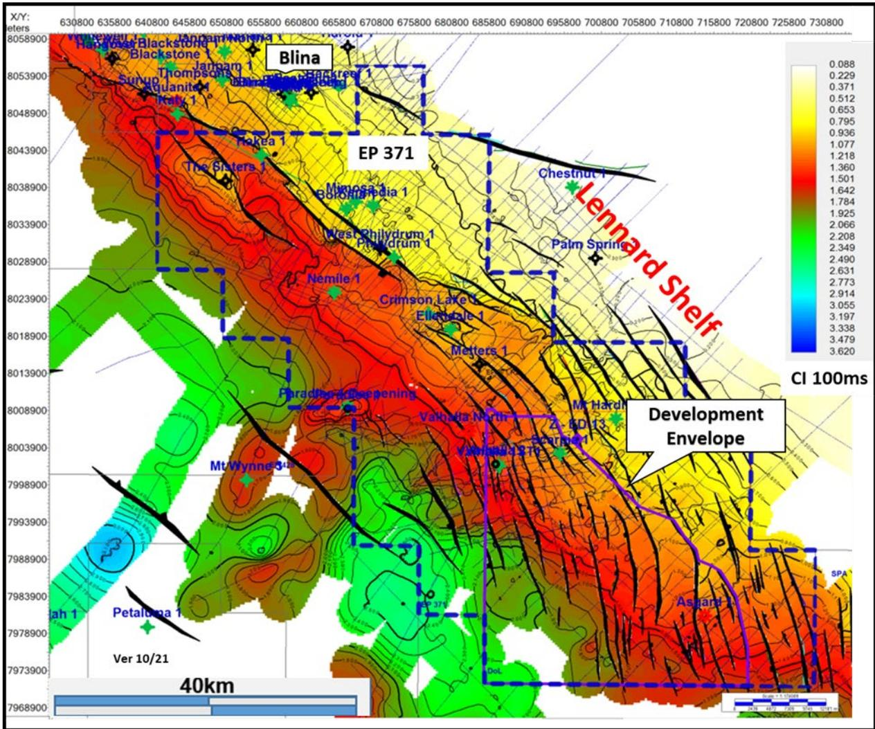
Figure 2-1: Regional Top Laurel Time Structure Map over EP 371 illustrating the deeper basin depocenter related to the underlying Fitzroy Trough to the southwest along with some of the established faulting within the DoL
