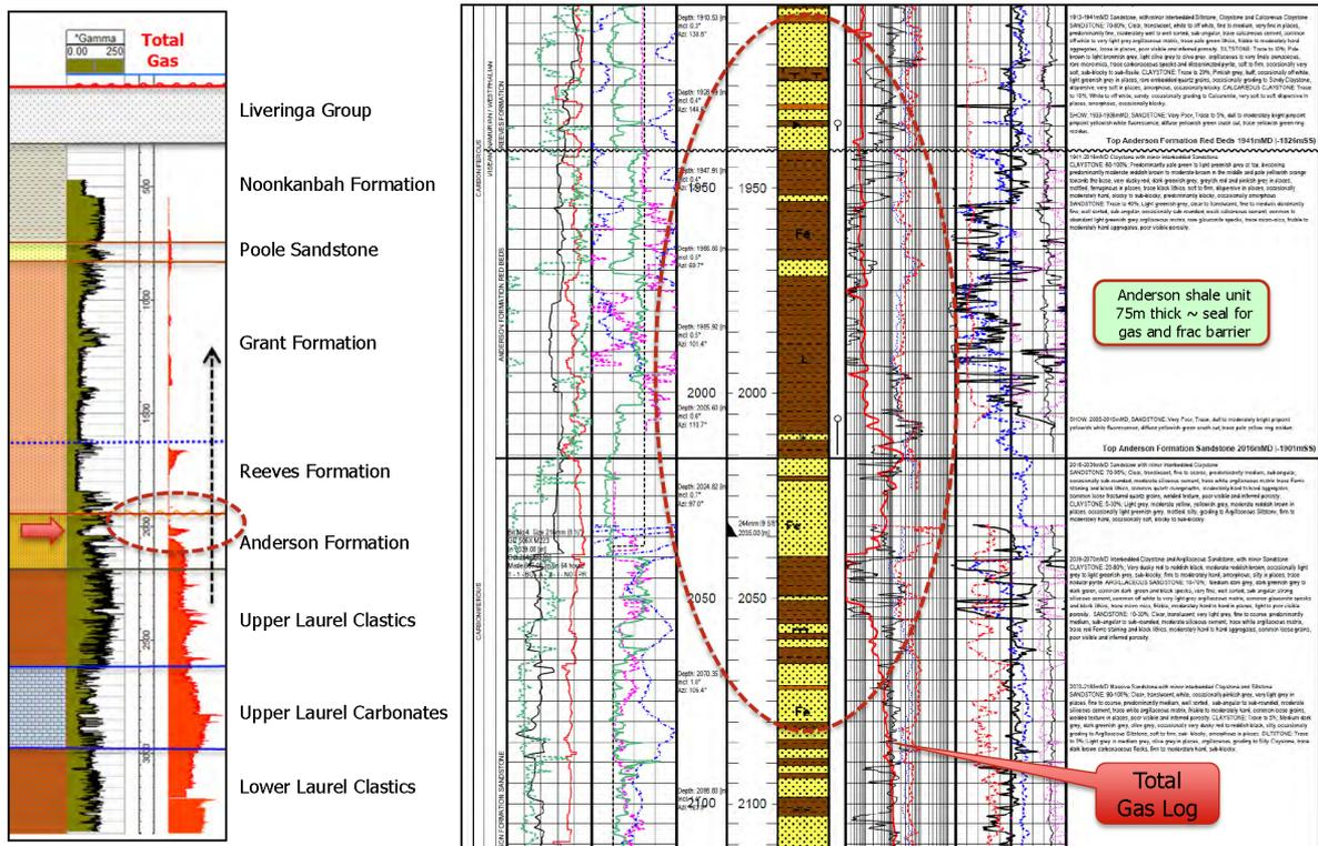
Figure 3-4: Composite well log for Valhalla North 1 showing the shale seal and the top of the gas section
