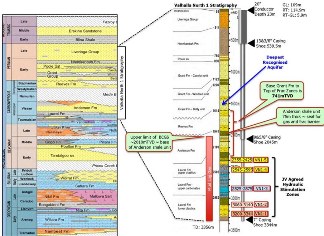
Figure 3-3: Valhalla North 1 stratigraphic section highlighting the Anderson Formation shale seal between the hydrocarbon bearing zones of the Anderson and Laurel Formations, and the Grant / Reeves sections above along with proposed hydraulic stimulation zones. Actual zones for the stimulations were deeper than the shallowest ones illustrated here
