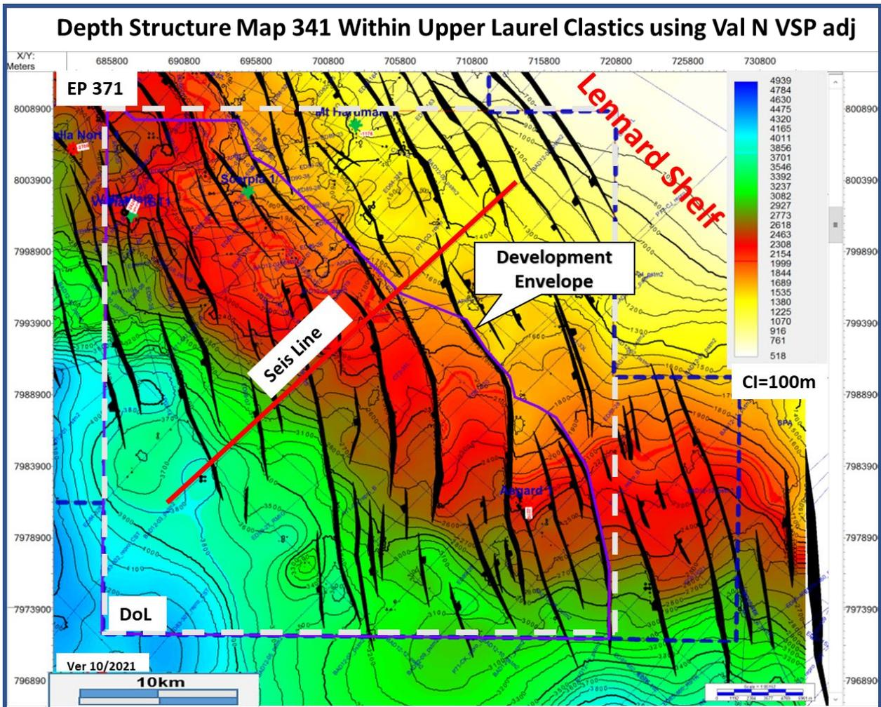
Figure 2-3: The 341 surfaces just above the Upper Laurel Carbonate is shown highlighting a number of downthrown normal faults stepping into the basin. The DoL is marked with the box. The location of the seismic line from Figure 2-2 is also marked
